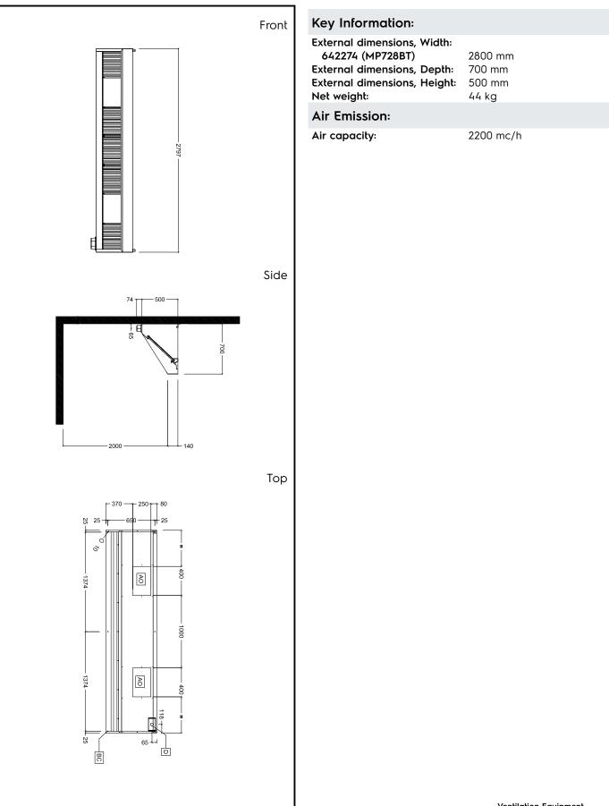
Ventilation Equipment 430 S/S Wall Hood+Filters 2800X700mm
